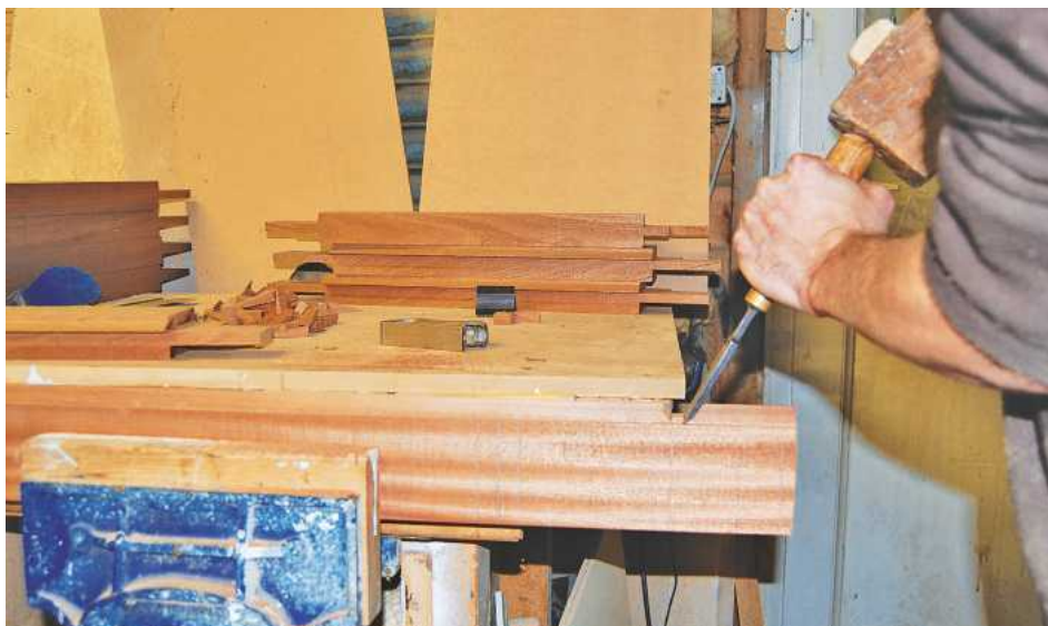
▲ Pic.8 Jason removing the waste from the tenon cheeks...
